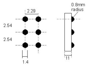
Fig.11 Dimensions of Braille Cell
