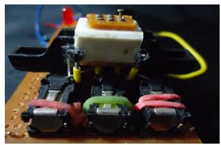
Fig. 10 Actuated Braille cell
