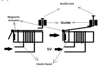
Fig.8 Braille cell representing actuation process
